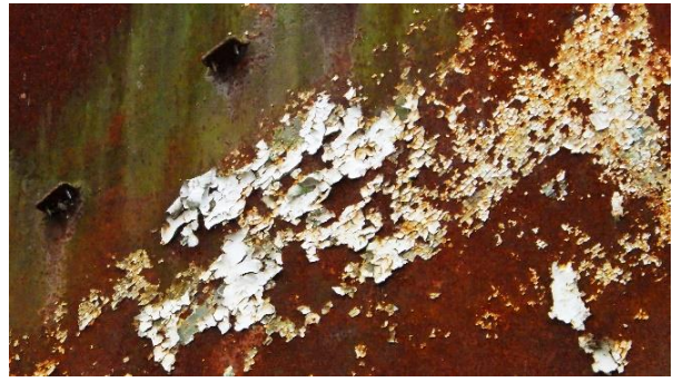
Sea Scout Wreck rust and peeling paint
